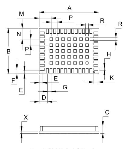
Figure 2-2 UM982 Mechanical Dimensions
