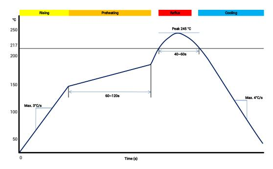
Figure 4-1 Soldering Temperature (Lead-free)
