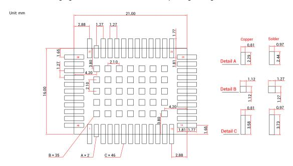
Figure 3-4 Recommended PCB Package Design
