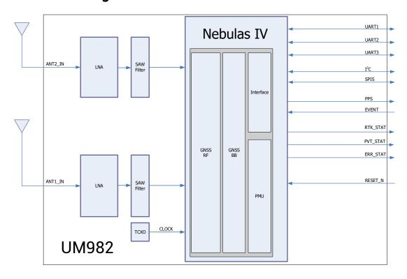
Figure 1-2 UM982 Block Diagram
