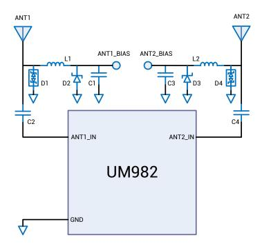
Figure 3-2 UM982 External Antenna Feed Reference Circuit
