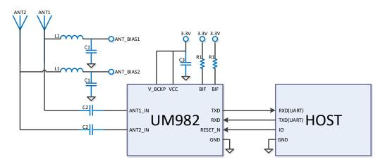
Figure 3-1 Recommended Minimal Design
