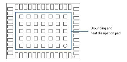
Figure 3-3 Grounding and Heat Dissipation Pad (Bottom View)
